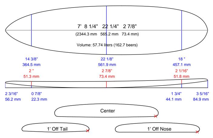
Measurements are center, one foot in and one foot back, over curve.
